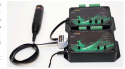
The above photo shows a single handheld trigger with LADC connected to a microMANTIS and a miniMANTIS. The controllers are connected together with an LADC cable and splitter. Note that only one power source is required as the microMANTIS (top) receives its power from the miniMANTIS via the LADC cable.
